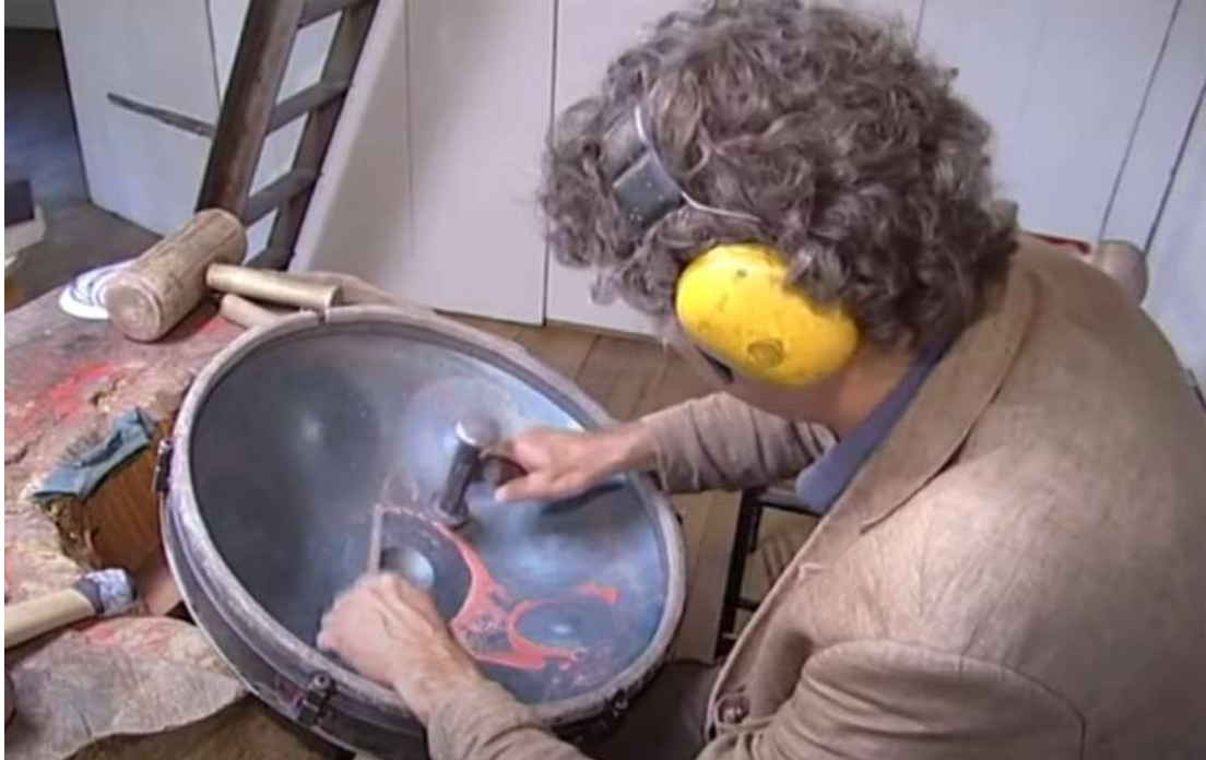
Figure 4.15 Rohner tuning the Hang in the 2006 documentary by Castan & Pagnon 2006. Screenshot by the author. 103
